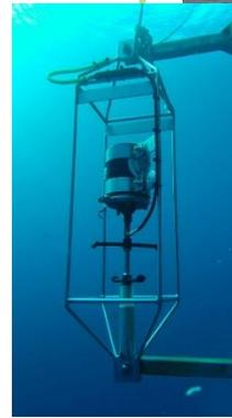
The **Falmouth Scientific Remote Coastal Reporter** is a turn-key system that provides transmission of real-time sensor data from remote areas to the Internet of Things (IoT) cloud for access by users around the world.
